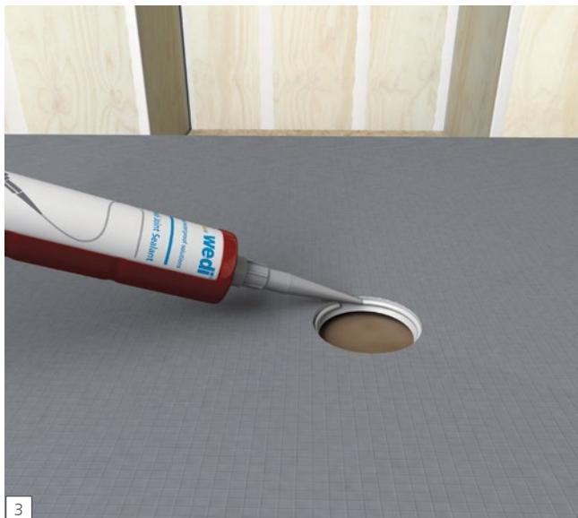
**EN** Set up a continuous 1/4" (6.4 mm) bead of wedi sealant along the top side of the wedi Fundos' valve groove profile. Optionally you can apply the bead on the underside of the main drain body's flange. This will help keeping sealant off the threads of the main drain body when it is inserted.
