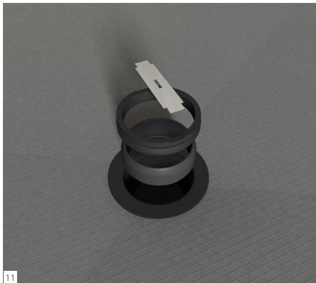
**EN** Tighten (squeeze) the rubber caulking gasket firmly with the caulking nut (use a flat headed screwdriver) and finally insert the plastic frame and strainer on top (without adhesive). The frame and strainer will be held in a grout joint only once tiling commences. Do not tighten the gasket prior to 60 minutes after the threaded drain part was sealed into the shower base.
